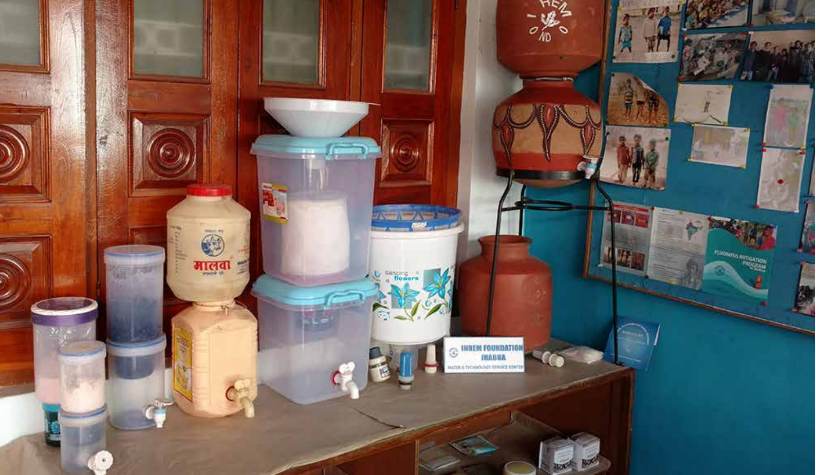
Change in design of water filters from clay to plastic to deal with breakage of clay pots | Source: INREM Foundation Website
